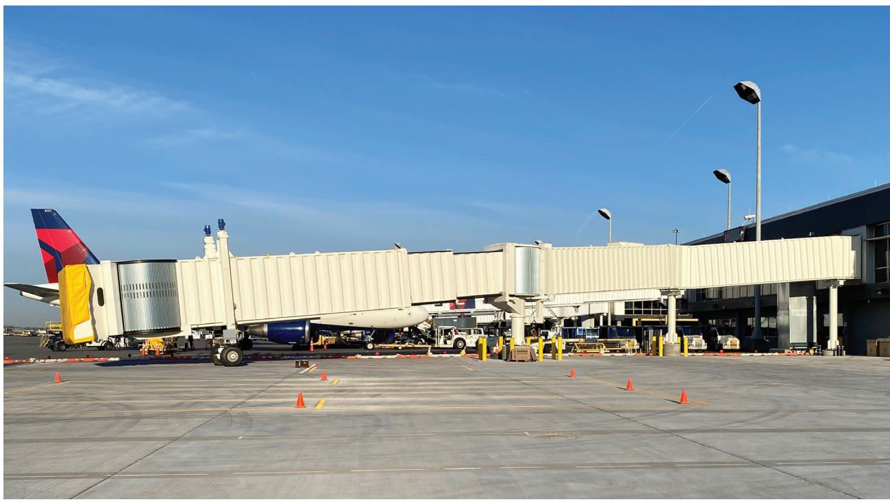
Two old passenger boarding bridges were diverted from the waste stream and modified to provide a necessary link from the work area to customs and immigration facilities during construction
